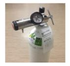
In either case the connecting mount to the flow meter should be checked for leaks. Usually a leak is audible on careful listening
